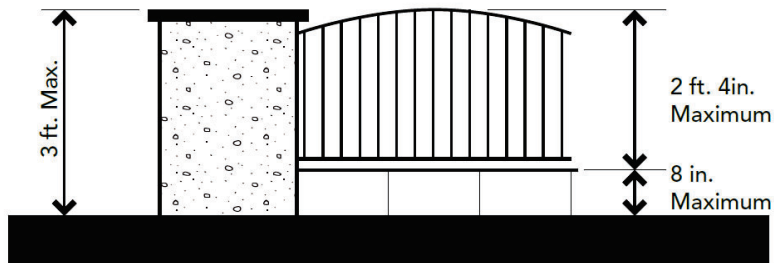
Figure 3-11 Fence in R-1 Zone
